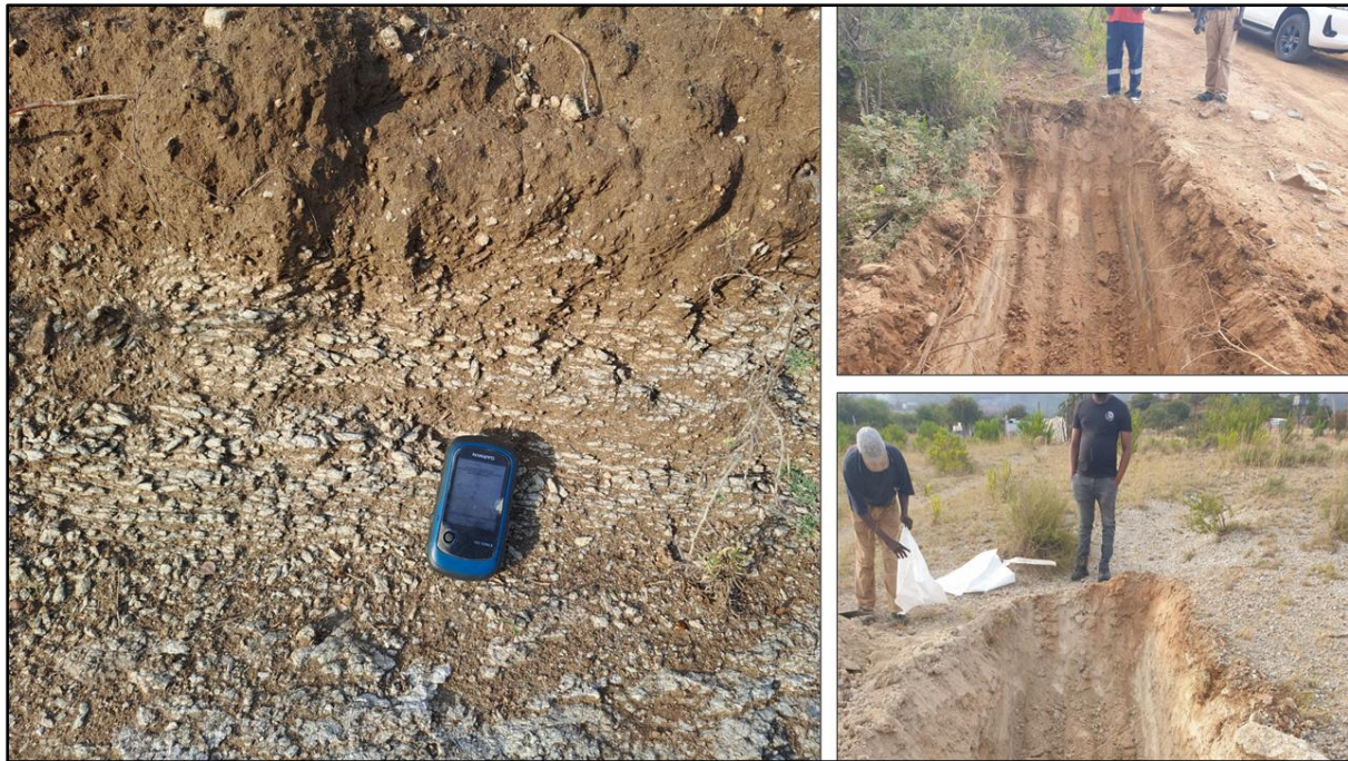
Figure 13: View of the identified shallow Glenrosa/Mispah, Coega and rocky outcrops soil forms.
